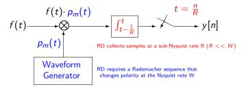
Generating a waveform that changes polarity at a high rate might be just as hard as building an ADC
